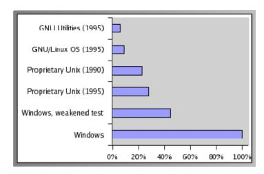
Fig 3. Failure Rates as Measured by Fuzz Tests
